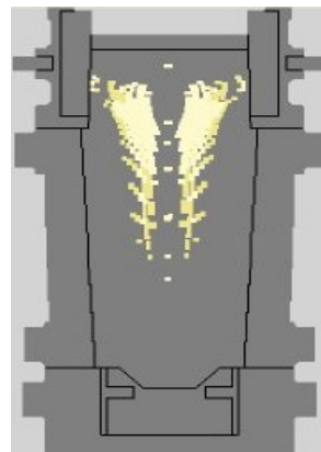
Figure 3. Macro segregation area and non destructive control results
